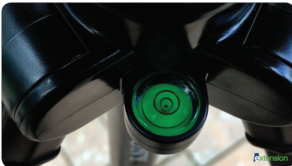
Make sure your camera is level before filming. Adjust your tripod legs so the bubble in the tripod's bubble level is centered.
